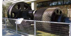
Gear used for deceleration of the feed roll from the Planetary Hot Rolling Mill. The mill had been used as main machinery at Nippon Yakin Kogyo for 30 years. Access / Kawasaki City or Rinko Bus (5 mins) from JR Kawasaki Sta. 1min walk from Kvoiku-bunka-kaikan mae stop
